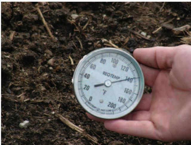
The most important diagnostic tool for composting manure and sludge is a long-stemmed (4 ft) thermometer. A compost pile that is properly assembled should warm to the 140 degree F range within three or four days.
