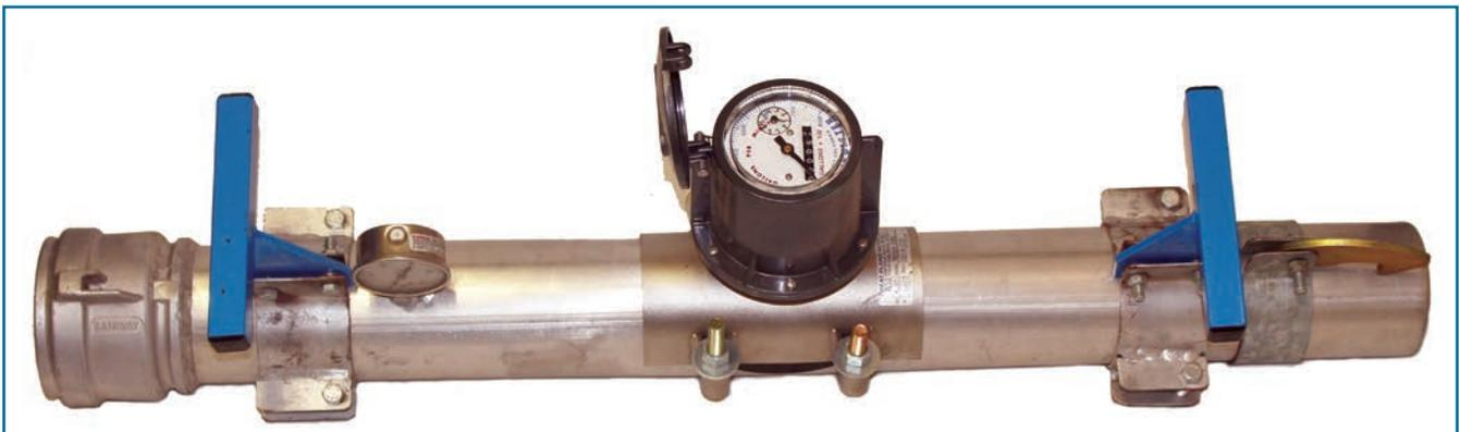
Figure 7. Portable propeller test meter equipped with a pressure gage, quick-connects and handles for insertion into existing water supply pipelines for measuring flow rates.
