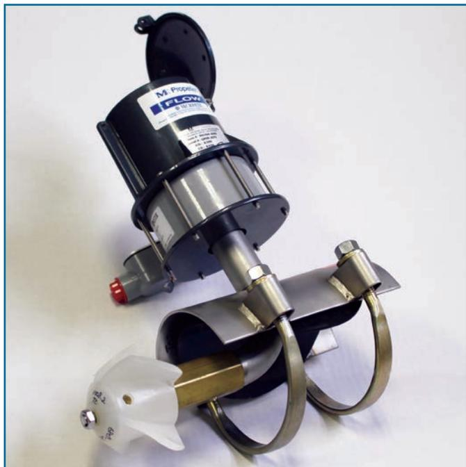
**Figure 8.** Saddle flow meter which can be installed into an existing pipeline by cutting a hole in the top of the pipe. Meter shown has an optional digital output for use with irrigation control and monitoring systems.
