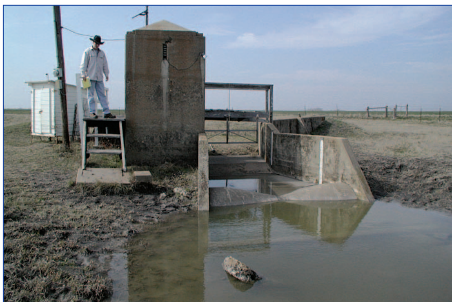
Figure 3. Field equipment to collect surface runoff.
